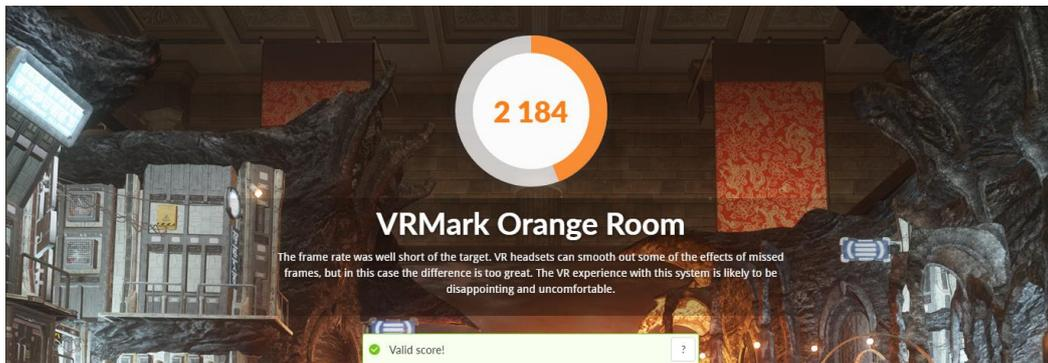
The ring graphic is a visual indication of VR-readiness. It shows how the system's average frame rate during the benchmark run compares with the target frame rate for the test. The ring is fully orange when the system's average frame rate meets or exceeds the target frame rate.
